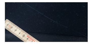
• Deep scratches over 25 mm that cannot be polished. This does not apply to the edge of the loading area.
